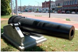
The facility cast its first cannon, a 7-inch Brooke rifle, in July 1863. The most common pieces produced at Selma were the 6.4-inch Brooke, which was just over 11 feet and weighed more than 10,000 pounds, and the 7-inch, 12-plus foot piece, weighing as much as 15,000 pounds. Selma is also believed to have cast 11 of the 11-inch Brooke smoothbore guns that weighed in excess of 20,000 pounds but completed and shipped only eight.
